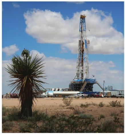
Compared with a previous well with a 17,935-ft lateral that was drilled in 18 days, a new well with an 18,325-ft lateral has been drilled by Latshaw Rig 10 in just 12.5 days. This time reduction was primarily enabled by eliminating a planned trip at 15,000 ft.
